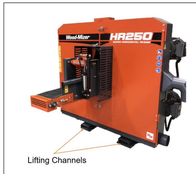
Lifting an unpacked machine
